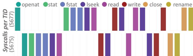
Fig. 3: Syscalls issued over time by RANSOMEXX's encryption threads to file F10573.bqt.vmdk.
